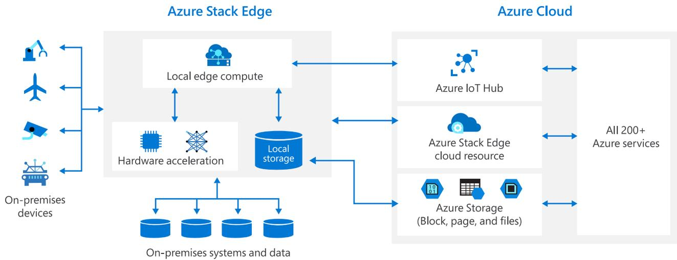
Azure Stack Edge combines IoT Edge and accelerated ML inferencing in a cloud-managed edge computing appliance delivered as an Azure service
